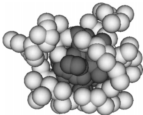
Figure 1. A snapshot of the collapsed equilibrium configuration of the diblock copolymer. The dark beads are type A monomers, and the light beads type B monomers.
